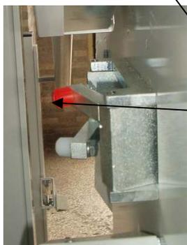
Levers for unclamping are at the backside of the platform
