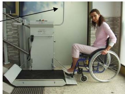
Close the barrier when on the platform. When the barrier is closed the ramps will automatically lift up. This is an additional safety feature that secures the wheelchair.
