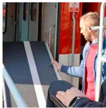
Perfectly adjustable thanks to the width-adjustable ramp (upper stop)
