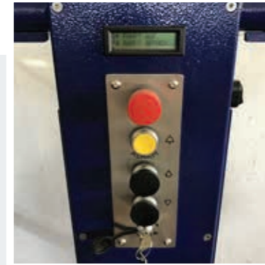
Control on the platform with stop and alarm button, as well as a display for status and fault indication
