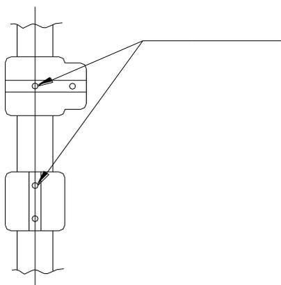
Make sure that that the screws in the center of the main tube are in line with each other before operating. If the screws are in the right postion, thighten them.
