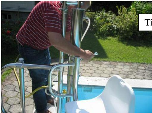
Tightening the seat bracket (seat height is adjustable)
